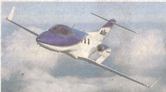
The HondaJet's unorthodox design places the engines above the wings.
