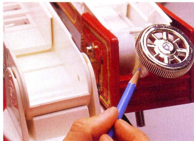
Following a DFMA design review by Hasbro engineers, the ladder assembly on the Tonka Talk n' Play Firetruck was redesigned in plastic, the number of components was reduced from 33 to 5, and assembly time dropped from 198 to 22 sec.
