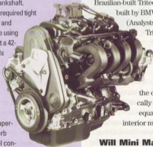
Chrysler's original 2.0L Neon engine strongly influenced BMW's engine designers for the Mini motor.
