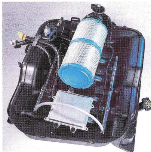
Siemens' induction module, aimed at a 2003-model V-8, combines air-intake, engine-control and fuel-delivery systems.
